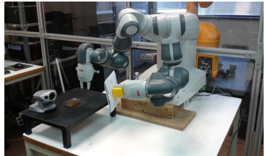
Implementation of a visual servo control in a bi-manual collaborative robot.
